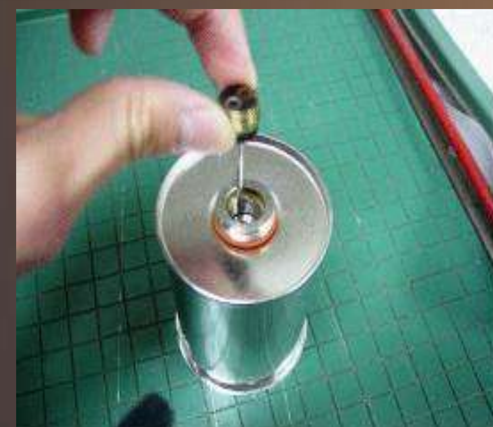
Pea puree sealed in can with thermocouple. Cans heated in steam at 104.4C, 112.8C, and 120.6C
